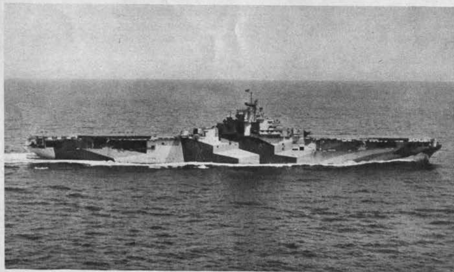
New spoon bow on U.S.S. Hancock looks clipper in beam view, flares out into broad, rounded platform at top. Bow and stern project beyond ends of flight deck.
